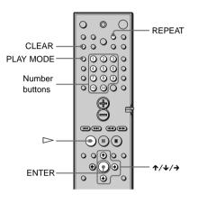
In stop mode, press PLAY MODE repeatedly until "PROGRAM" appears on the front panel display.
